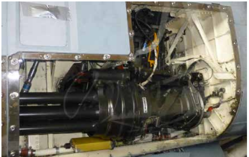
Top and center: Views of the M61A1 gun on the Tomcat. Right: A closer view of the gun drive motor.
