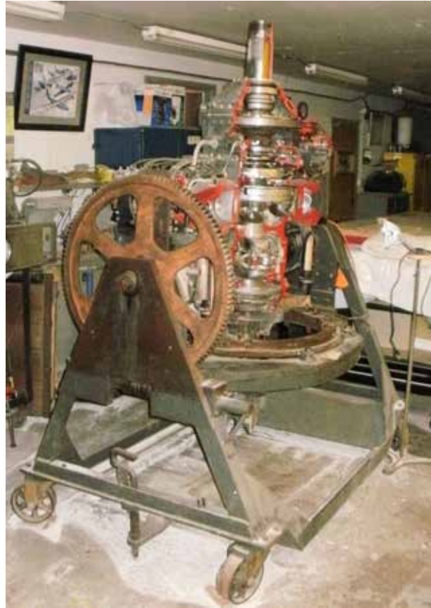
Far Right: A view of the cutaway section. Above: An oblique view showing the large gear wheel for rotating the engine through an 180 degree arc.
